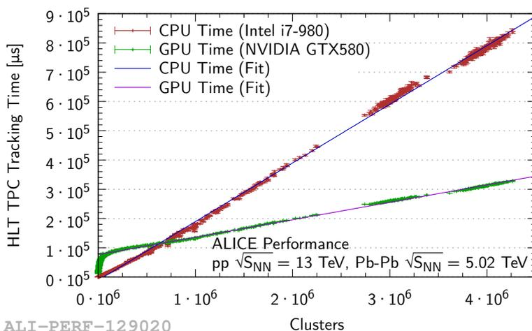
Time needed for track finding on a CPU compared to a GPU as a function of the number of TPC clusters
